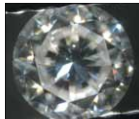
Fish eye: Grey reflections of the girdle just inside the table, due to incorrect girdle thickness, table % and pavilion angle. Gut grade poor to fair.
